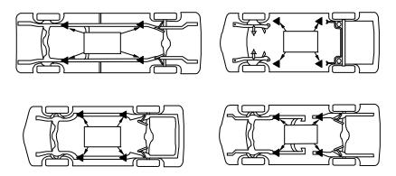
Refer to the manufacturer's specific vehicle lifting points. Some vehicles display these points on a label inside the right front door lock face or are identified by triangle shape marks on the vehicle's undercarriage, reference SAE J2184.
