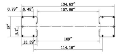
**STEP 8:** Use the existing holes in column base plate as a guide for drilling the 3/4" diameter holes into the concrete. Drill the anchor holes <u>only</u> for ONE column, installing anchors as you go. You will install anchors in second column after the cables, hoses, and floorplate are installed.
