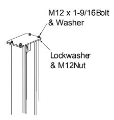
**STEP 7**: Position the columns facing each other **134-5/8**" outside base plates. Square the columns by measuring diagonally from corner points on base plates (within 1/4").
