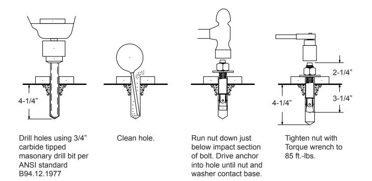
**STEP 9:** Using a level, check column for side-to-side plumb and front-to-back plumb. If needed, use horseshoe shims provided by placing shims underneath the base plate and around the anchor bolt. This will prevent bending the column bottom plates (Shim thickness should not exceed 1/2"). Tighten 3/4" anchor bolts to **85 ft-lbs.** of torque.
